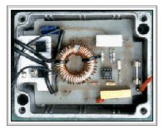
The step up converter built from a kit. It starts from just four volts snd outputs s regulated 14 volts to the battery
