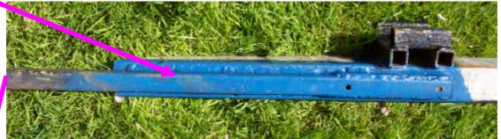
A bar was also welded to the other end of the extension piece to make it easier to control the tower during lifting and lowering. This also got a coat of paint to stop it from rusting.
