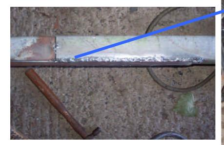
I tested the tower frame to make sure it was strong enough to hold the wind turbine. I did this by suspending the tower on two stands at each end of the tower and then I stood in the middle and bounced to simulate the wind which will try to do the same.
