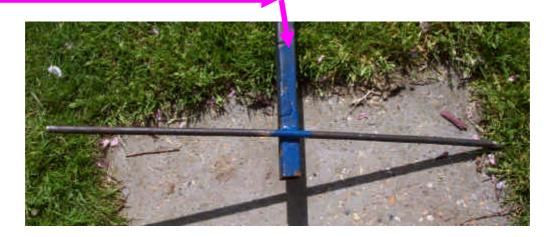
The top part of the tower needs some means of attaching the YAW bearing from the wind turbine frame. To do this I decided to use more scaffold clamps as they our very strong and are designed to cope with large forces such as the ones the wind turbine will exert. These also got welded to the top of the tower. But this time I got a professional welder to do this as it is imperative that this all holds up to the forces of the wind turbine blades pushing and vibrating on and down the tower.
