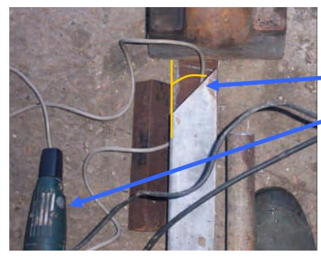
As you can see this is one piece of the U tubing with the 45 deg angle cut into it with the angle grinder on the left of the photo.
