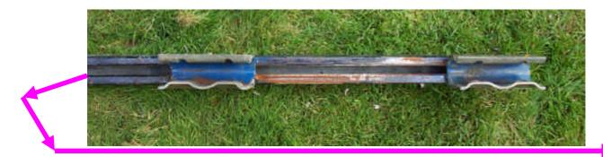
I also asked the professional welder to weld the YAW bearing which is smaller then the clamps can hold into a 1 meter long piece of scaffold. This scaffold can now be clamped by the scaffold clamps.
