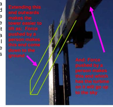
Here you can see the tower in its erected state, you can also see the extended leaver which is made from the same box section that
