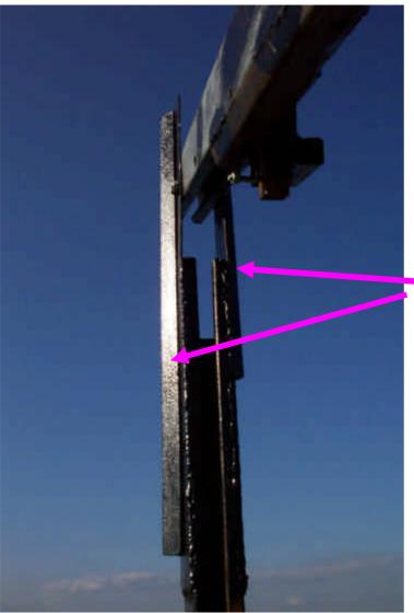
I continued to test the tower by tying to erect the top piece without any thing on it. I found that it was very difficult and that my hinge was simply not rigid enough to take the top tower piece. So I had to add some sort of extra bracket and I came up with the idea of using angle iron to stop left to right movement. But only one side was welded the hinge could still be tightened up.
