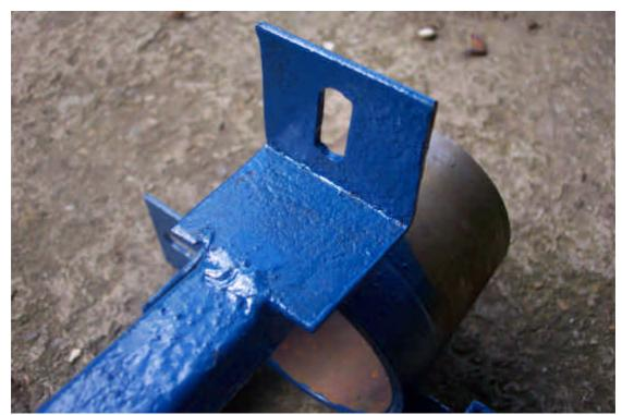
hold the laminates for the PMG. These slots where cut using a milling machine which makes them accurate and smooth.
