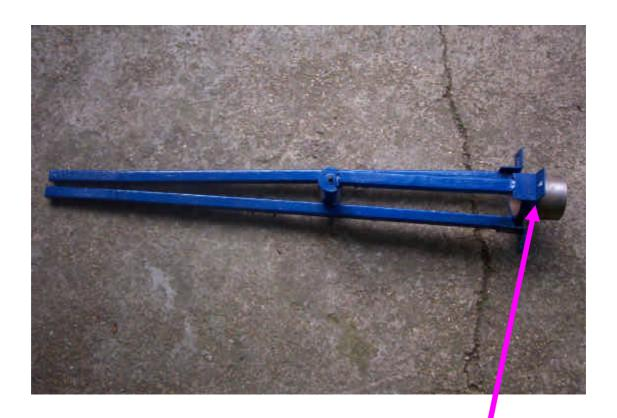
The main bearing of the PMG will sit in this pipe here.
