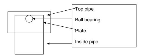
I used some pipe that wasn't a perfect match so I had to use the metal lathe to make the inside diameter wider so that the pipe would fit inside it.
