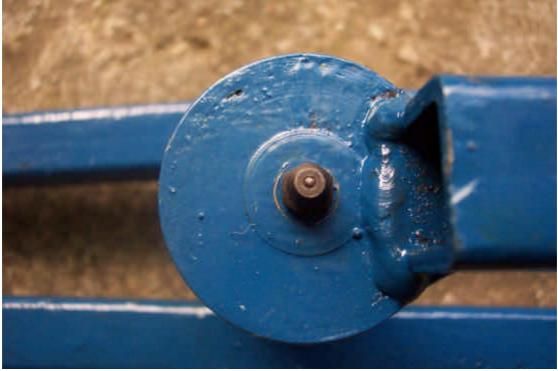
will make it a lot easier to pump grease into the bearing which will increase the life time of the bearing by reducing ware.
