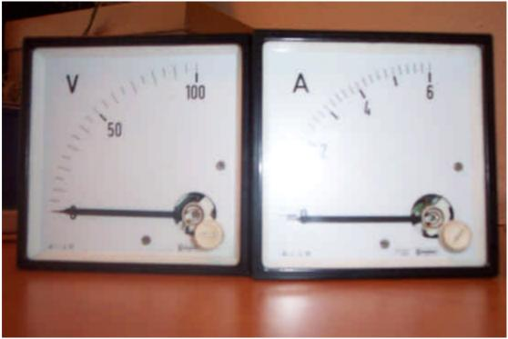
I was also able to get two meters from the company where I got the wire. The one on the left measures volts dc and the one on the right measures amps. Mr Bigin will install these as he sees fit but they where part of the specification to have a clear indicated of power.
