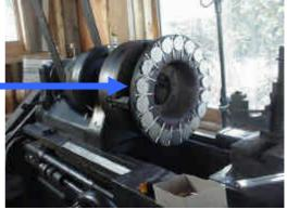
As you can see the top part of the PMG is made from a car disk brake which is machined on a lathe to take the Neo magnets which are the strongest magnets that are made.
