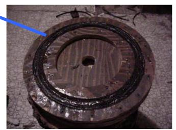
This picture shows what are called the laminates which are just simple strips of metal that are curved to form a circle and then ether placed in a ply wood former or are cast in fibre glass. These help to pull the magnetic power (flux) from the magnets through the coils which are placed on top of them.
