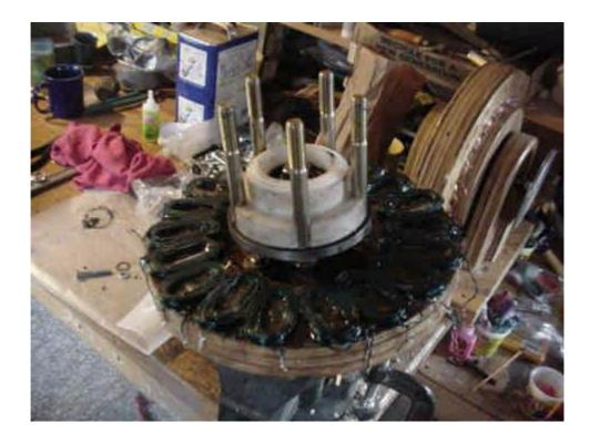
Once the coils have been wired up and the magnetic rotor is placed on the extended wheel studs then the PMG is completed and ready for testing:
