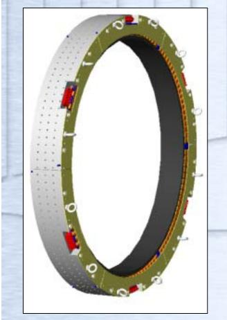
Direct drive generators offer maintenance free operation and highest efficiency at the expense olf large volume, mass, cost
