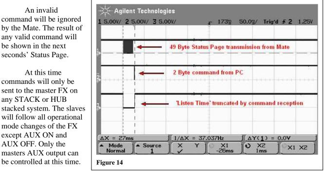
It is also important to note that a users pressing any of the Mate buttons interrupts both Status page transmissions and listen time for 2 seconds. A button press will cease all PC communications until no button has been pressed for 2 seconds.
