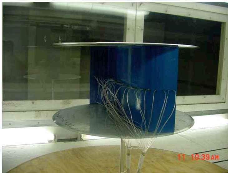
Figure 5. The wind turbine without the spanwise slots
