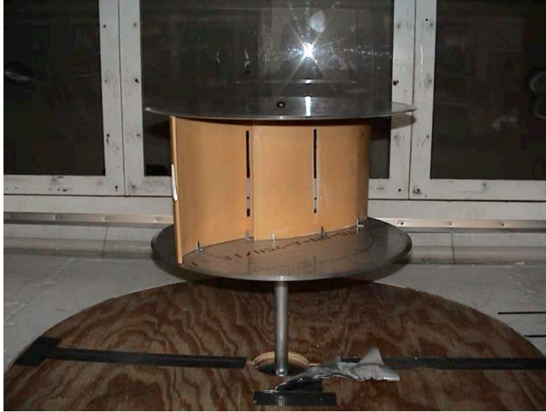
Figure 6. The wind turbine with the spanwise slots.
