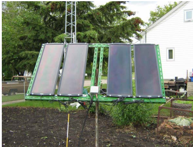
Illustration 1: Home made angle iron solar panel frame
