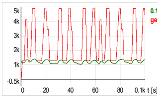
Fig. 14 Alternator Speed Profile and Voltage
